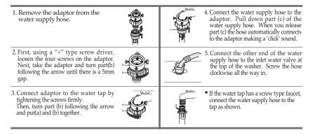
**NOTICE** After completing connection, if water leaks from the hose, then repeat the same steps. Use the most conventional type of faucet for water supply. In case the faucet is square or too big, remove the spacing ring before inserting the faucet into the adaptor.
